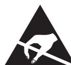
LA SCHEDA SIM E' SENSIBILE ALLE SCARICHE ELETTROSTATICHE, PER NON DANNEGGIARLA SI RACCOMANDA DI USARE LE PRECAUZIONI DEL CASO
